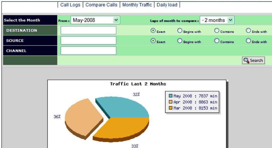
The final report is the Daily Load, which can show the call volume per hour over the course of the day. You can then drill down into the calls for a specific time frame.
