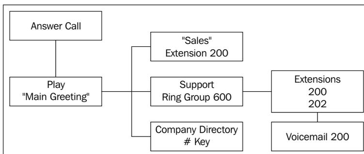
To set up IVR, select **IVR** from the left-hand navigation menu within the PBX Configuration tool. On the first screen, select the button to create a new IVR. The IVR creation page is broken up into general settings for this specific IVR and a section for keypresses and actions on the button.
